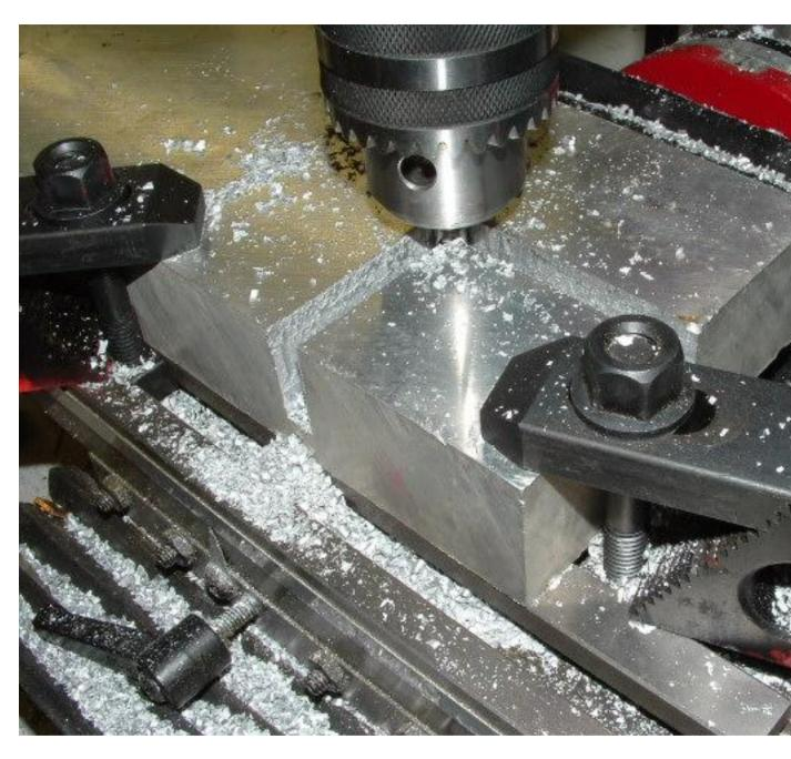
The billet is a little tall so I'll have to mill it to clear the inside of the body. Then I'll locate where the axle will be and drill for that which will tell me how much room for a fuel t ank I have. About twenty seven hours so far and most of that on the machine.
